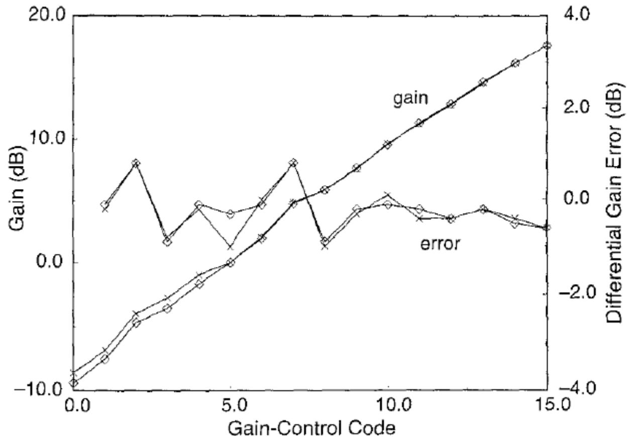
**Figure 4: Amplifier gain and gain error.**
