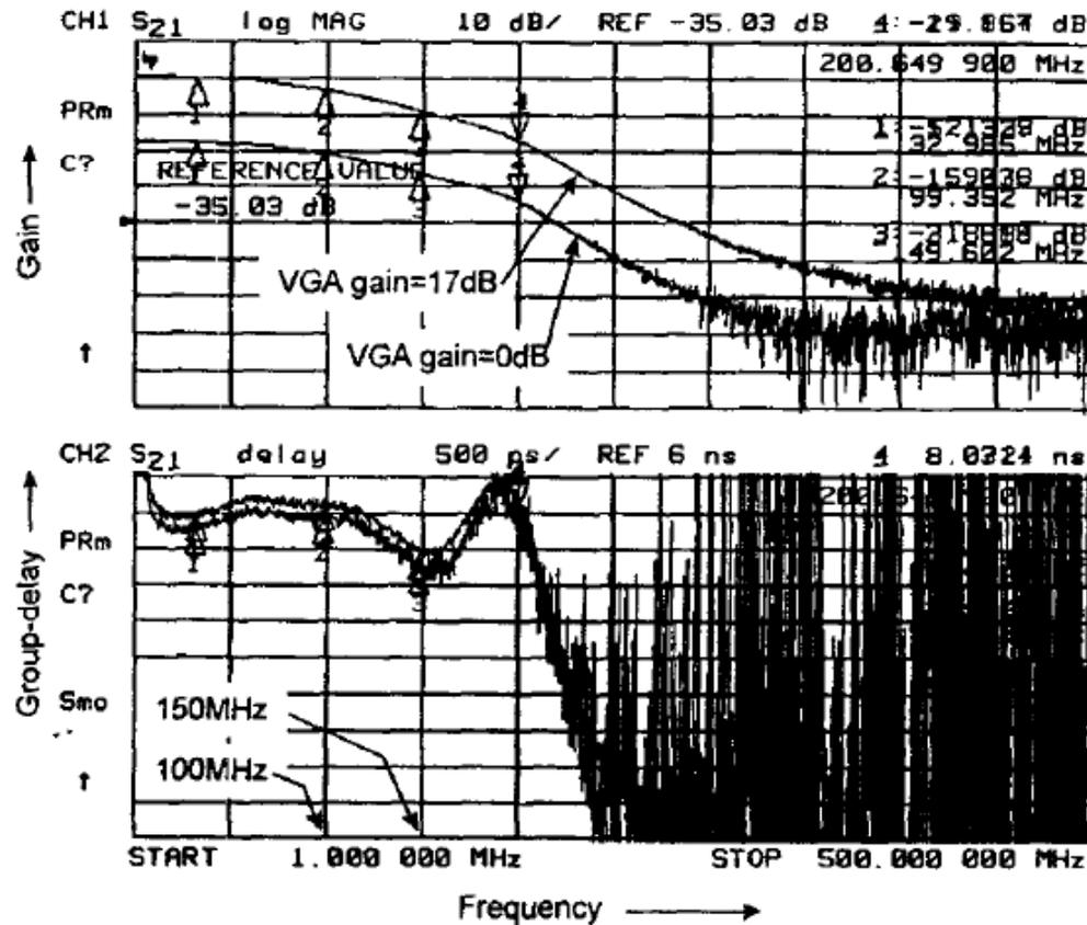
Figure 23.2.5: VGA operation.
