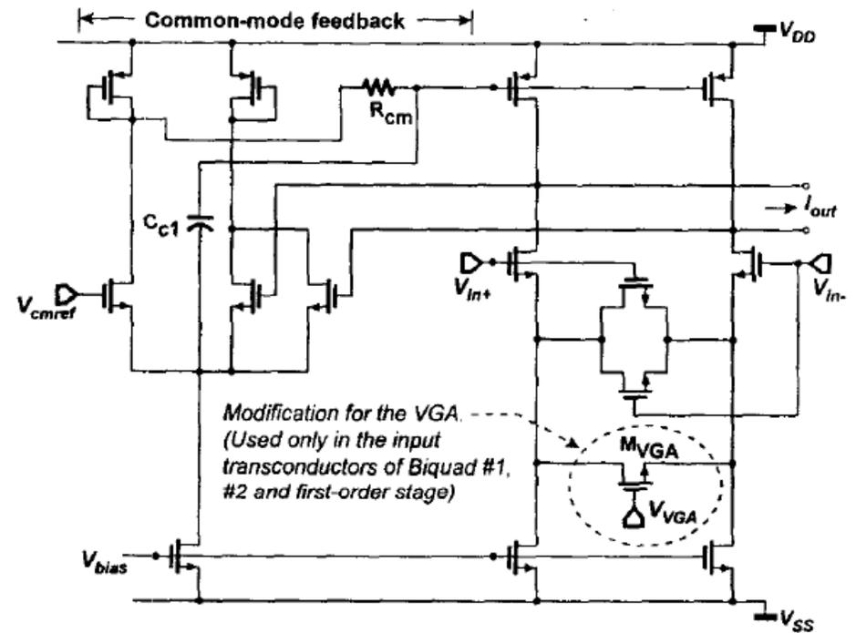
Figure 23.2.3: Complete transconductor.
