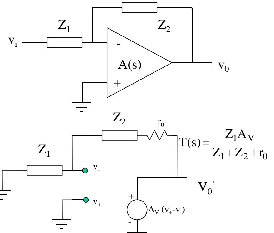
$$\frac{V_o}{v_i} = \left( \frac{V_o'}{v_i} \right) \frac{Z_1 + Z_2}{Z_1 + Z_2 + r_0} = -\frac{Z_2}{Z_1} \left[ \frac{1 - \frac{r_0}{A_V Z_2}}{1 + \frac{Z_2 + r_0}{Z_1}} \right]$$
