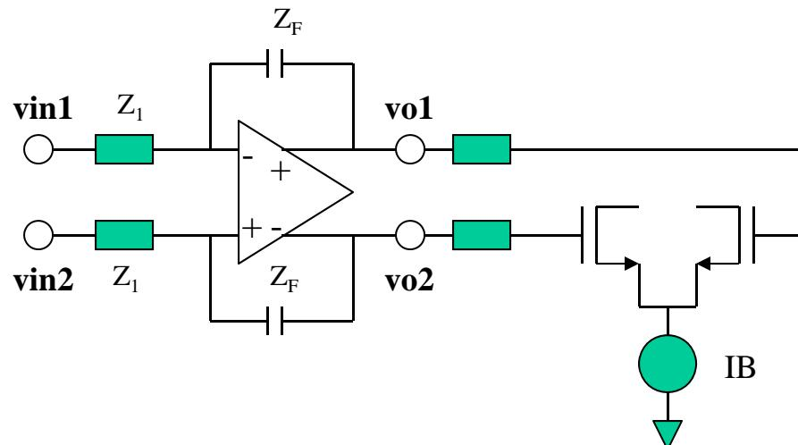
Common-mode offsets can impact the performance of the following stages
