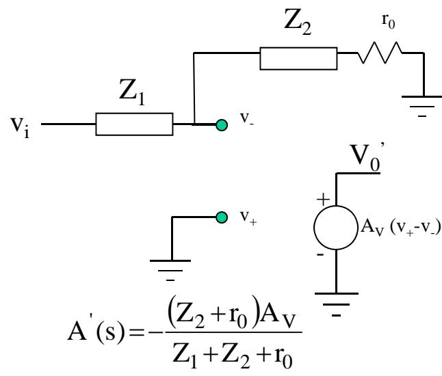
$$\frac{V_o'}{v_i} = -\frac{(Z_2 + r_0)A_V}{1 + \frac{Z_1 A_V}{Z_1 + Z_2 + r_0}}$$
