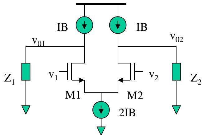
$$CMRR = \frac{A_{dd}}{A_{dc}} \cong \frac{g_{m1} \left( 1 + \frac{Z_1}{Z_2} \right)}{Y_s \left( 1 - \frac{g_{m1} Z_1}{g_{m2} Z_2} \right)}$$
