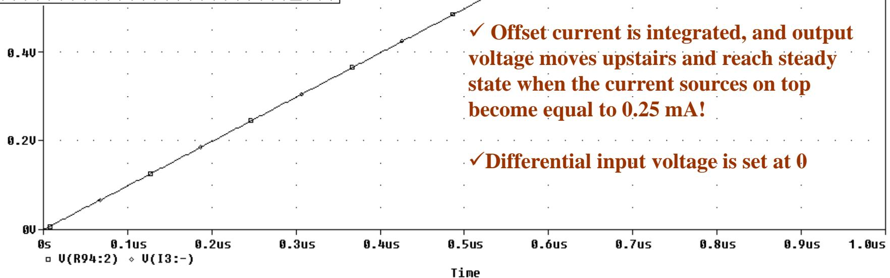
✓ Offset current is integrated, and output voltage moves upstairs and reach steady state when the current sources on top become equal to 0.25 mA!
