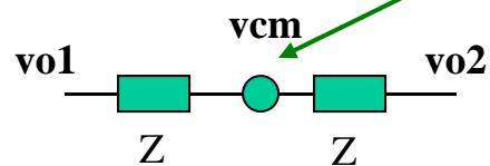
$$v_{cm} = \frac{v_{01} + v_{02}}{2}$$
