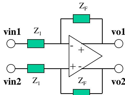
➤ A common-mode feedback loop must be used:
