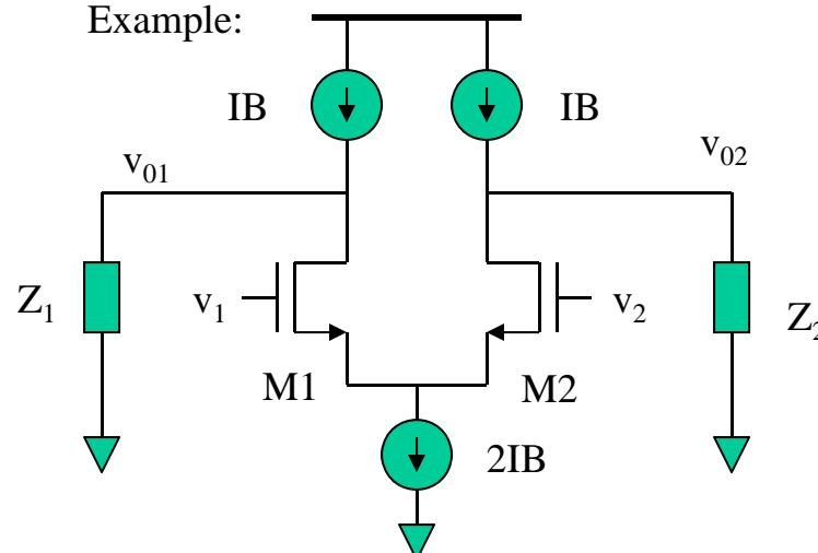
$$v_{01} = \frac{g_{m1}g_{m2}Z_1}{g_{m1} + g_{m2} + Y_s} \left[ \left( 1 + \frac{Y_s}{2g_{m2}} \right) v_{id} - \left( \frac{Y_s}{g_{m2}} \right) v_{ic} \right]$$
