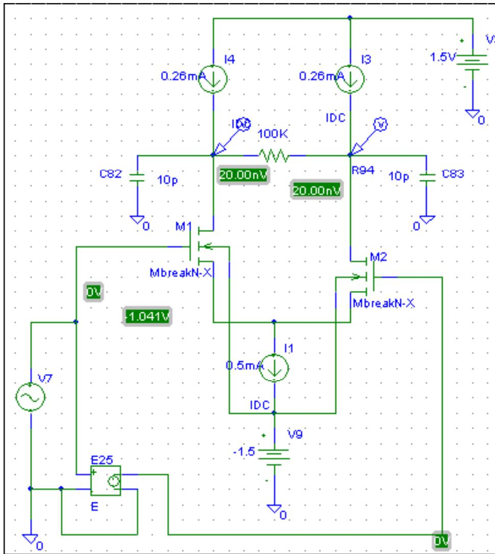
✓ Common-mode current offset of 0.01 mA per side is added on purpose
