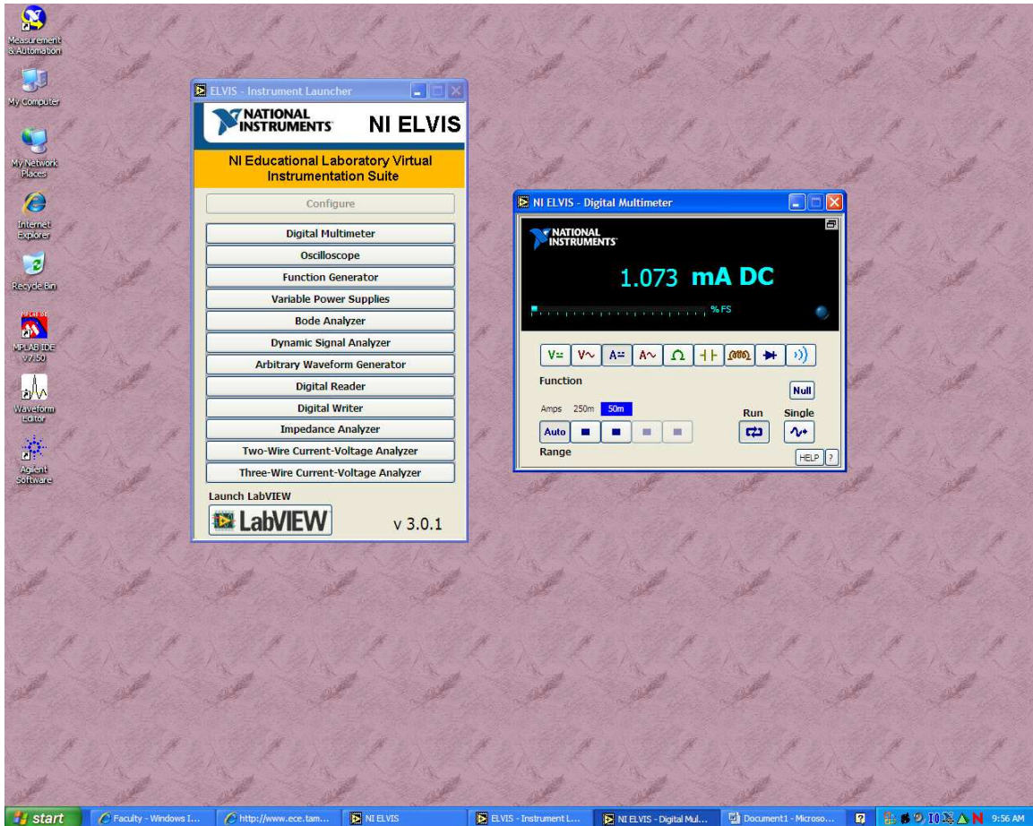
Figure 2.5: DC Current Measurement
