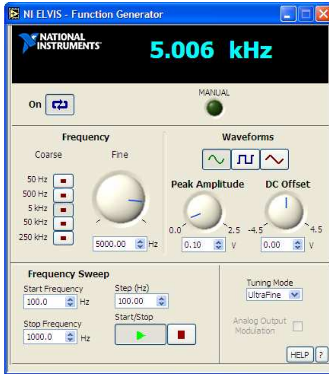
Figure 2.8: NI ELVIS Function Generator window
