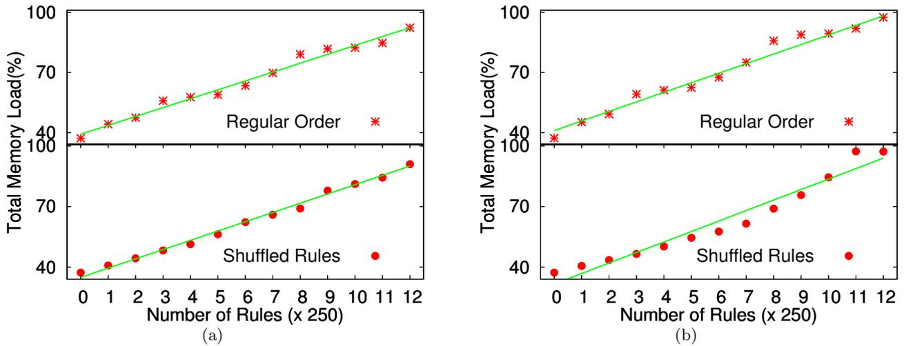
Figure 5: Linearity of memory consumption in different search algorithms as the number of activated rules increases: a) AC-bnf-aq; b) Lowmem.
