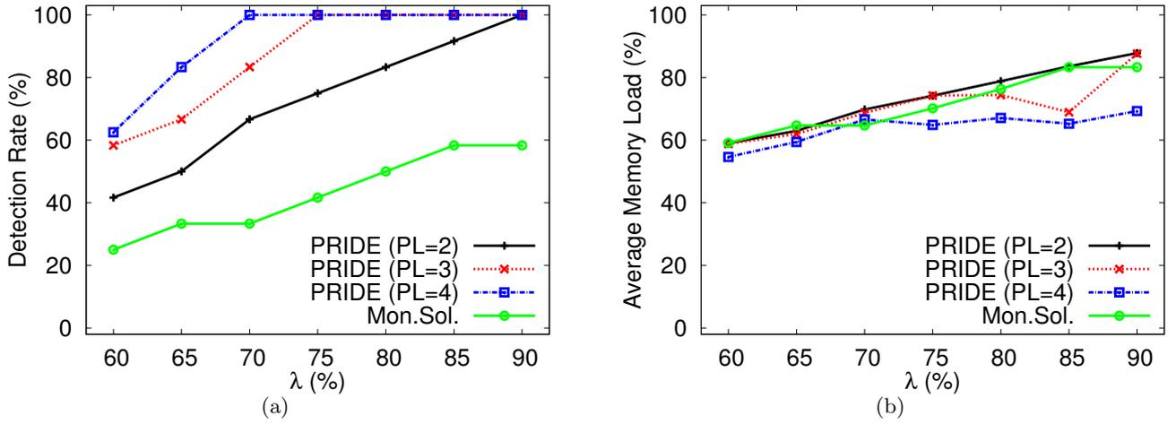
Figure 9: 12-module configuration: effect of  $\lambda$  and PL on a) Intrusion detection rate, and b) Average estimated memory load.
