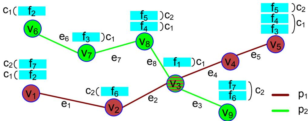
Figure 4: An example graph for a mesh network, consisting of 9 nodes and 8 links. As shown, two paths  $p_1$  and  $p_2$  are present. The nodes run different configurations of Snort, e.g., node  $v_5$  runs Snort functions  $f_3, f_4$  and  $f_5$ , which require preprocessors  $c_1$  and  $c_2$ .
