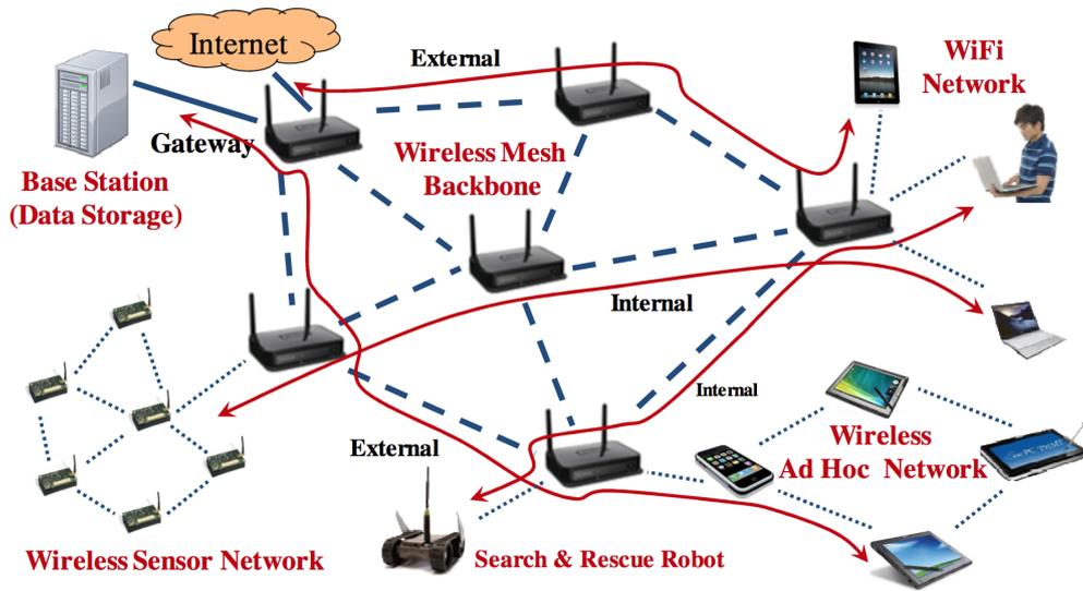
Figure 1: A typical mesh network providing network services for a variety of users.
