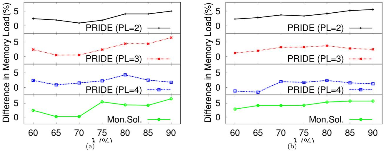
Figure 10: The difference between estimated and actual average memory load: a) 6-Module configuration, and b) 12-Module configuration.
