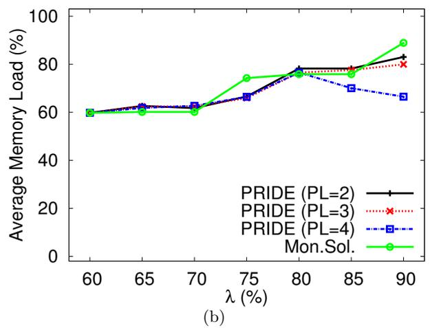
Figure 8: 6-module configuration: effect of  $\lambda$  and PL on a) Intrusion detection rate, and b) Average estimated memory load.
