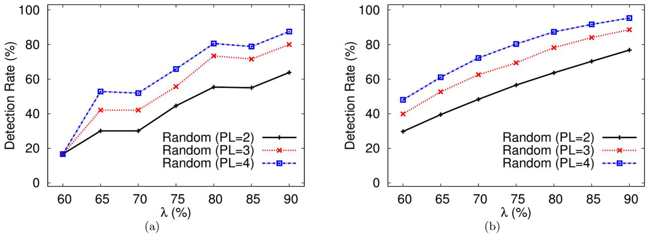
Figure 13: Distributed approach based on random module selection: effect of  $\lambda$  and PL on the intrusion detection rates in a) 6-Module Configuration, and b) 12-Module Configuration.
