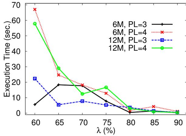
Figure 11: ILP solver execution time for different modularizations, path lengths and memory thresholds.
