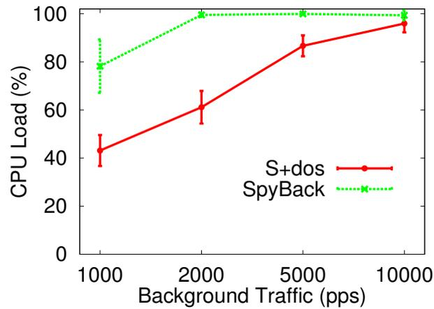
Figure 3: The effect of Snort configuration and traffic rates (packets per second) on CPU utilization.
