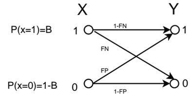
Figure 1: An abstract model for intrusion detection.
