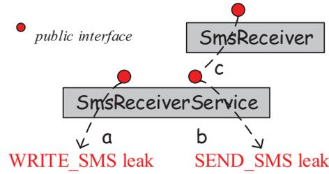
Fig. 6: Permission leak paths in Mms application.
