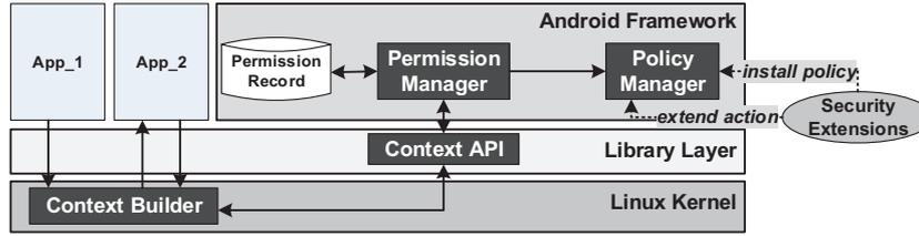
Fig. 1: Architecture of Context-Sensitive Permission Enforcement Framework.
