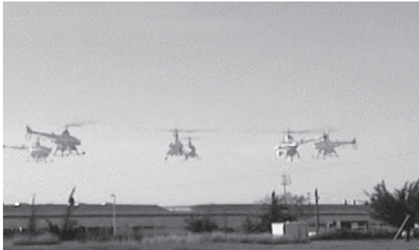
Figure 21.10 Superimposed time-lapse images of an autonomous helicopter performing a very difficult “nose-in circle” maneuver. The helicopter is under the control of a policy developed by the PEGASUS policy-search algorithm. A simulator model was developed by observing the effects of various control manipulations on the real helicopter; then the algorithm was run on the simulator model overnight. A variety of controllers were developed for different maneuvers. In all cases, performance far exceeded that of an expert human pilot using remote control. (Image courtesy of Andrew Ng.)
