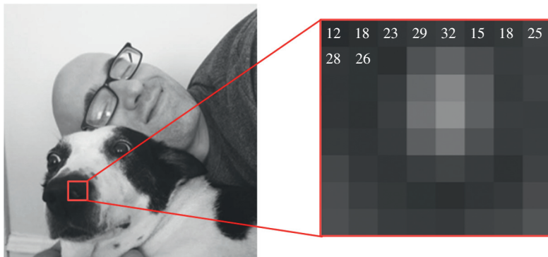
Fig. 4.25 An 8-bit grayscale image consists of pixels, each taking a value between 0 (black) and 255 (white). To visualize individual pixels, a small 8 \times 8 block from the original image is enlarged on the right.
