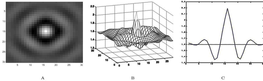
**Fig. 4. An Inversed DoG filter** The filter (i.e., the connection weights) of the central neuron is shown in log scale. **A.** A 2D plot of the filter. **B.** A 3D mesh plot of the filter. **C.** The plot of the central row of the filter. Note the multiple concentric rippling tails.
