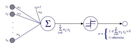
• The tunable parameters are the weights  $w_0, w_1, ..., w_n$ , so the space H of candidate hypotheses is the set of **all possible combination of real-valued weight vectors**:
