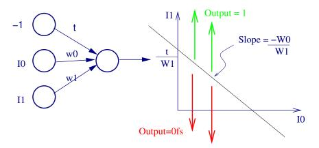
Perceptrons can only represent linearly separable functions.
