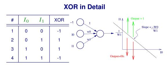
$W_0 \times I_0 + W_1 \times I_1 - t > 0$ , then output is 1:
