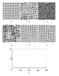
• Synthesize texture based on spectral histogram from observed image. Use of Gibbs sampler to reduce differences in SH.
