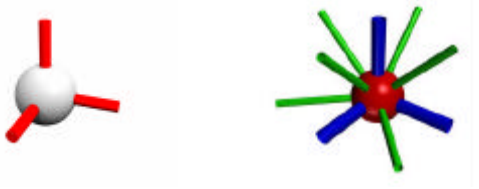
Figure 1. Vertices in a 3-connected and 9-connected EVDS. The bars show potential links to neighboring vertices.
