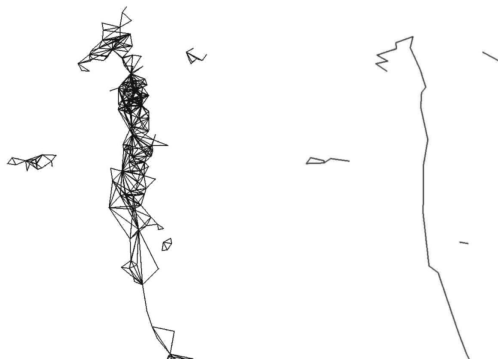
Figure 8. a) The connectivity graph for Figure 5. LBs in the same connected component are grouped in an LBC. b) The major threads from a.
