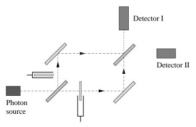
If we slide the phase shifter following output port 0 into the path, then its effect can be described by  $T_0(a|0\rangle + b|1\rangle) = -a|0\rangle + b|1\rangle$ . Similarly, if we slide the other phase shifter into the vertical path, then it has the effect  $T_1(a|0\rangle + b|1\rangle) = a|0\rangle - b|1\rangle$ .
