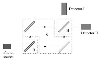
Our mirror devices operate as unitary operators on the state space  $\mathbb{C}^2$ . The behavior in then determined by  $HSH|0\rangle$ . By definition, we get
