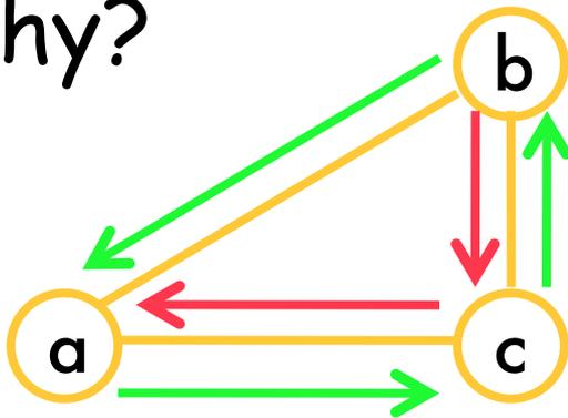
when tour created by going around the MST is adjusted to remove duplicate nodes, the two red edges are replaced with the green diagonal edge
