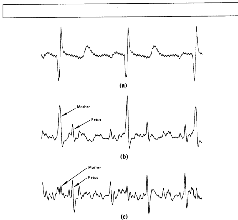
Figure 8. Result of fetal ECG experiment (bandwidth, 3-35 Hz; sampling rate, 256 Hz): (a) reference input (chest lead); (b) primary input (abdominal lead); (c) noise canceler output.
