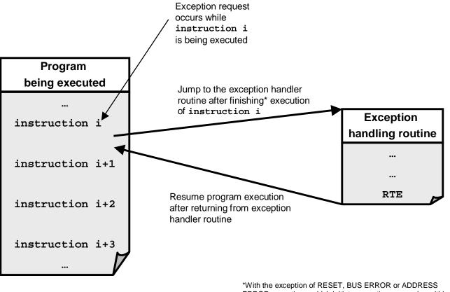
\*With the exception of RESET, BUS ERROR or ADDRESS ERROR exceptions, which initiate exception processing within two clock cycles
